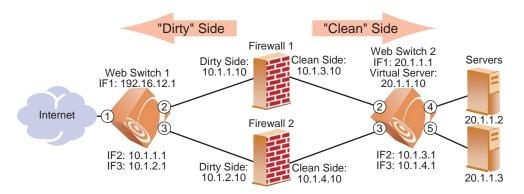
Figure 13-8 Basic FWLB Example Network
